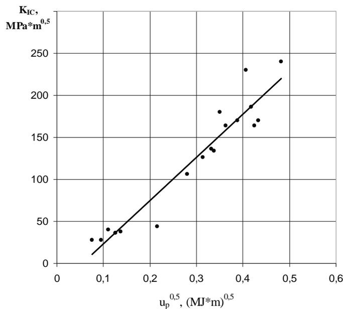
Fig. 2. The relationship between  $K_{IC}$ , and  $\sqrt{u_p}$
